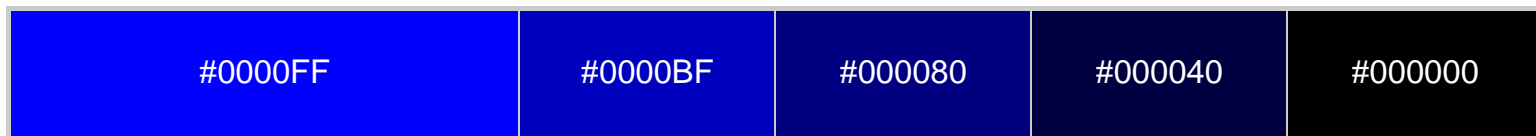
Figure: Demonstration of decreasing the brightness of pure blue in steps of 25%
